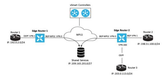
Edge Router 1 imports the source IP address of Router 1, 192.0.2.0/24 to VPN 0 on Edge Router 1. Thus 192.0.2.0/24 is a route leaked into VPN 0. Edge Router 2 imports the source IP address of Router 2, 198.51.100.0/24 and the source IP address of Edge Router 3,203.0.113.0/24 to VPN 0 on Edge Router 2.
