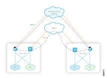
Each Cisco IOS XE Catalyst SD-WAN device supports up to eight TLOCs, allowing a single Cisco IOS XE Catalyst SD-WAN device to connect to up to eight different WAN networks. This capability allows path customization for application traffic that has different needs in terms of packet loss and latency.
