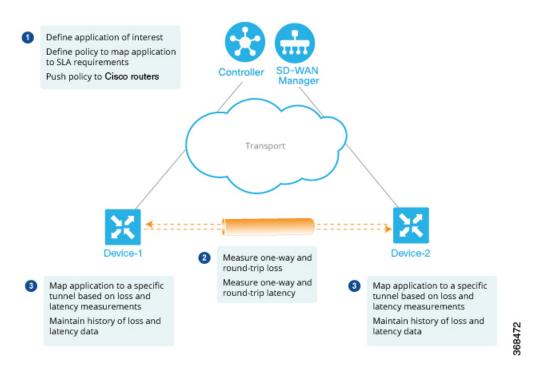
To create a data policy based on the Layer 7 application itself, configure the Cisco Catalyst SD-WAN Application Intelligence Engine (SAIE) flow with a centralized data policy. With the SAIE flow, you can direct traffic to a specific tunnel, based on the remote TLOC, the remote TLOC, or both. You cannot direct traffic to tunnels based on SLA classes.
