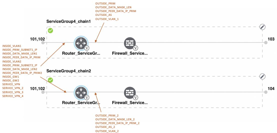
**Figure 23: Shared–Cisco vEdge Router VNF in First Position**
