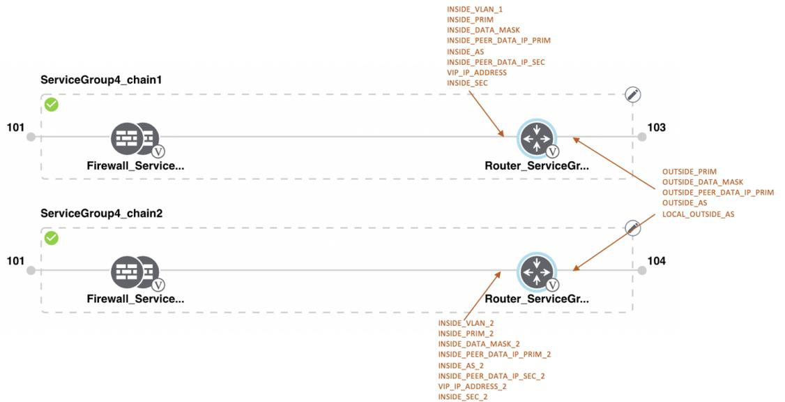
Figure 27: Shared-Cisco CSR1000V VNF in Last Position
