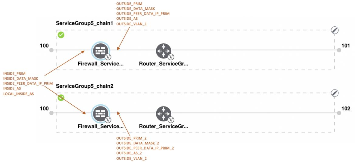
**Figure 30: Shared-ASA v VNF in First Position**
