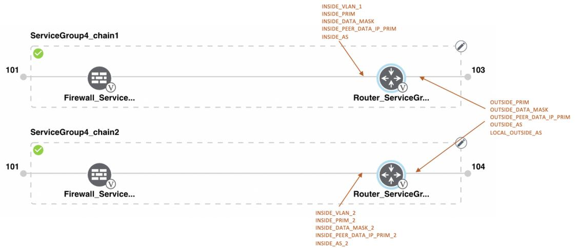
Figure 26: Shared-Cisco CSR1000V VNF in Last Position
