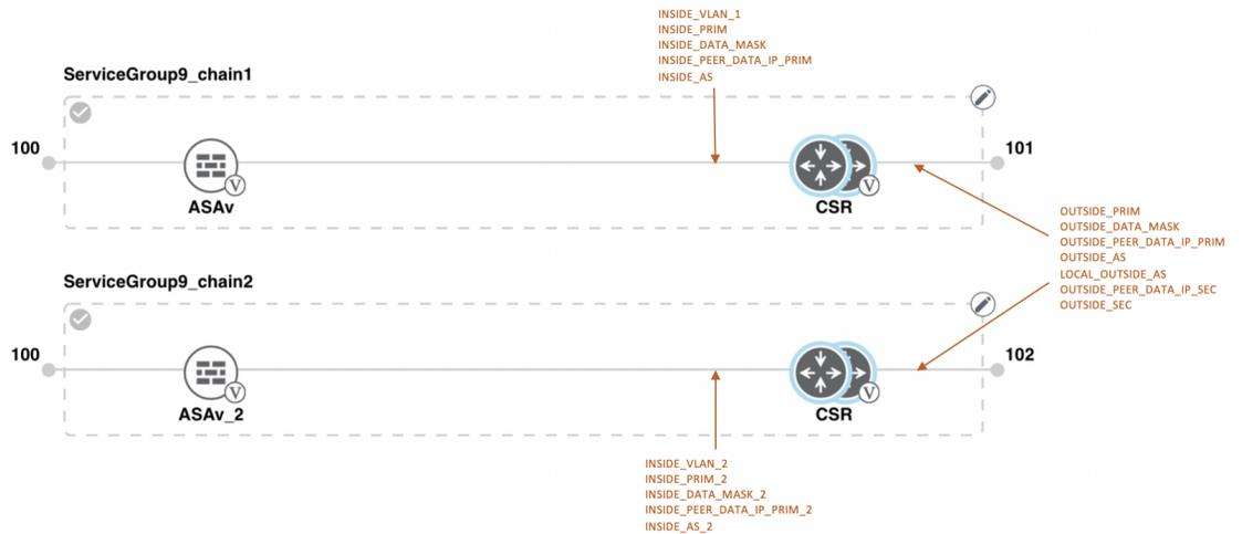
Figure 25: Shared-Cisco CSR1000V VNF in Last Position
