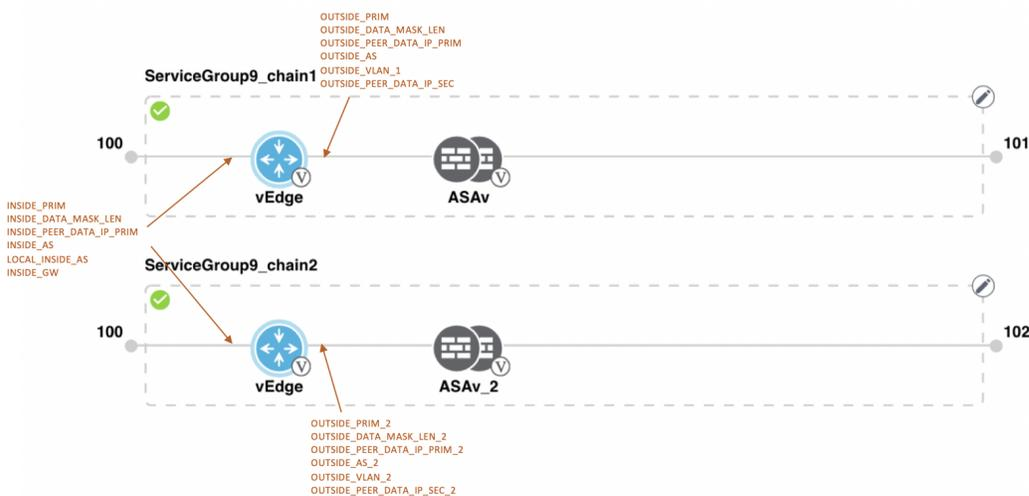
**Figure 21: Shared–Cisco vEdge Router VNF in First Position**
