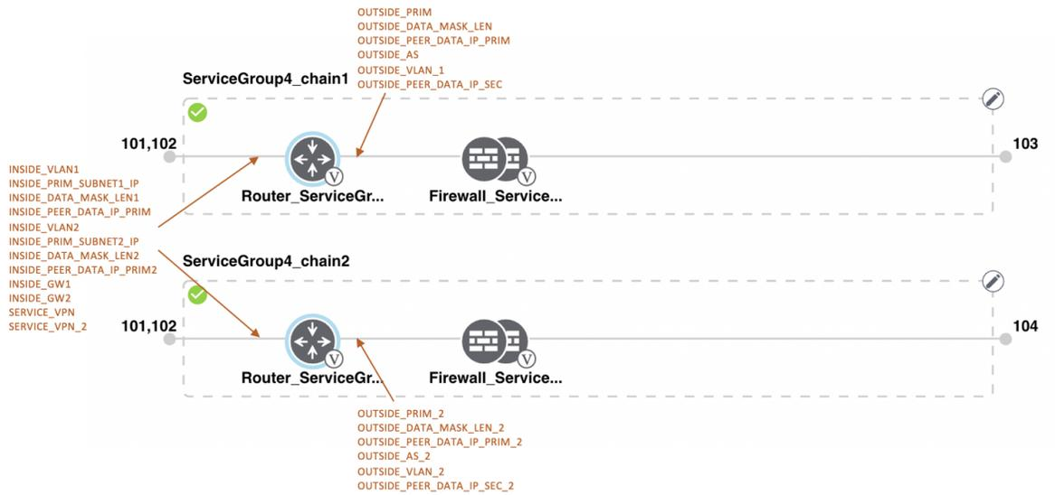
Figure 24: Shared-Cisco CSR1000V VNF in Last Position
