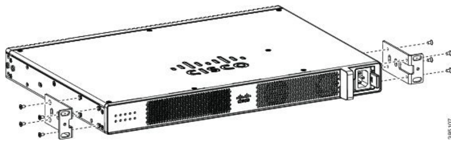
Figure 3: Bracket Installation for Back Mounting
