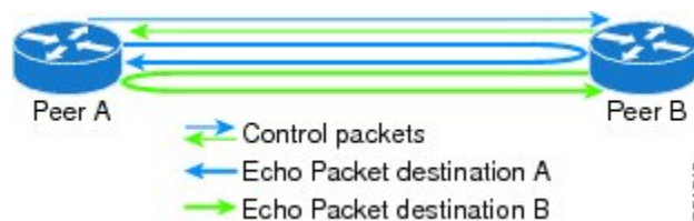
Figure 2: BFD Asynchronous Mode With Echo Packets
