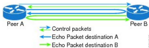
Figure 2: BFD Asynchronous Mode With Echo Packets
