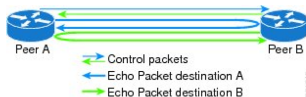
Figure 9: BFD Asynchronous Mode With Echo Packets
