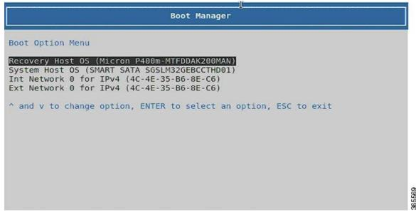
The router is recovered by using the recovery image in the hard disk recovery partition.
