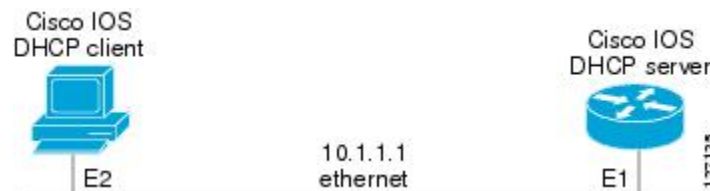
Figure 2: Topology Showing DHCP Client with GigabitEthernet Interface
