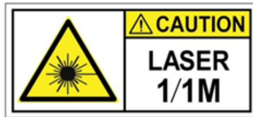
Figure 10: Class 1M Laser Product Label
