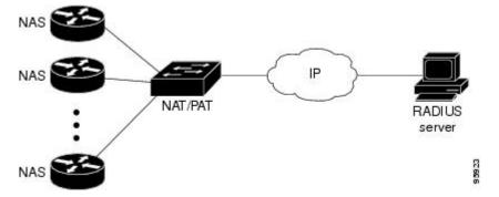
RADIUS servers normally check the source IP address in the IP header of the RADIUS packets to track the source of the RADIUS requests and to maintain security. The NAT or PAT solution satisfies these requirements because only a single source IP address is used even though RADIUS packets come from different NAS routers.
