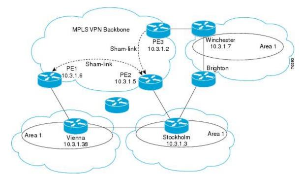
The following output shows the forwarding that occurs between sites from the standpoint of how PE-1 views the 10.3.1.7/32 prefix, the loopback1 interface of the Winchester CE router in the figure.
