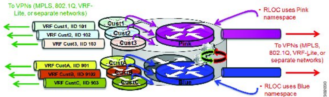
Figure 6: LISP shared and parallel models may be combined for maximum flexibility.
