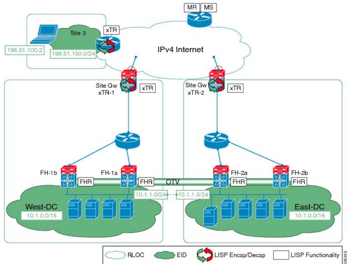
Multiple Layer 3 hops can exist between the FHR and the site gateway xTR when deploying the LISP ESM Multihop Mobility feature. You can insert non-LISP devices like firewalls and load-balancers into the data center.
