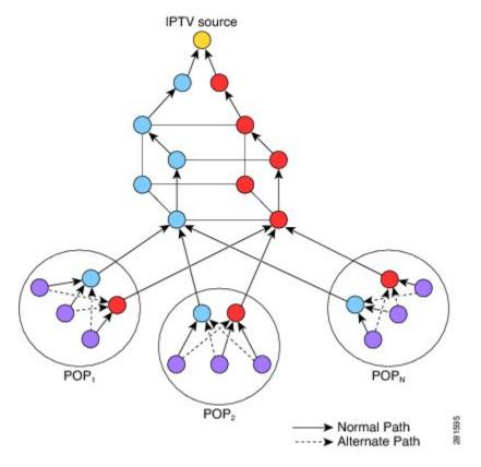
When a routing failure occurs, for example due to a link failure in the blue path, the red upstream router in the red plane becomes the primary upstream router to reach the source. This link to the router then becomes the RPF interface, and the copy of the multicast stream being received on the link is accepted and forwarded to the downstream links.
