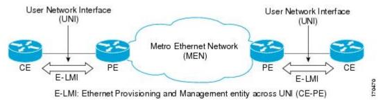
LMI also provides the status of Ethernet virtual circuits (EVCs) in large Ethernet MANs and WANs to the CE. Specifically, Ethernet LMI notifies a CE device of the operating state of an EVC and the time when an EVC is added or deleted. Ethernet LMI also communicates EVC and user network identifier (UNI) attributes to a CE device.
