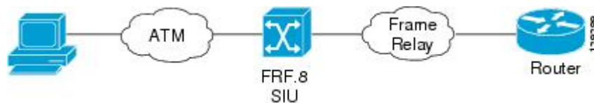
Figure 1: Frame Relay-to-ATM Interworking
