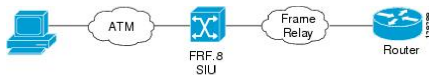
Figure 11: Frame Relay-to-ATM Interworking
