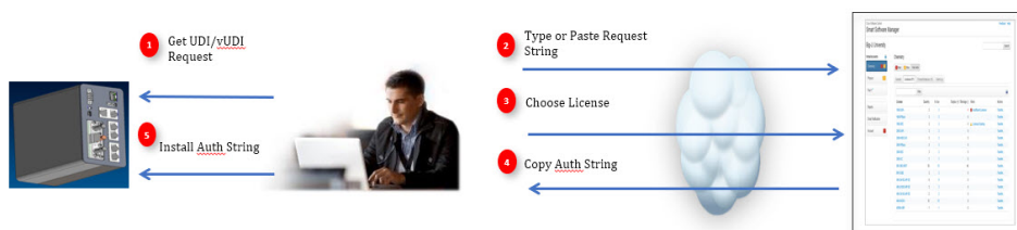
Figure 1: SLR Installation Flow
