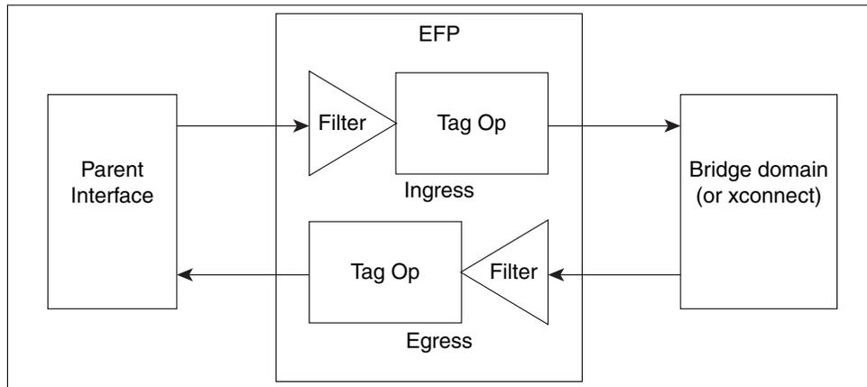
An EFP subinterface is configured to specify which traffic on ingress is vectored to that EFP. This is done by specifying a VLAN ID or QinQ tagging to match against on ingress. All traffic on ingress is compared to each EFP's matching criterion, and processed by that EFP if a match occurs. The processing performed by an EFP can change VLAN IDs, add or remove VLAN tags, and change ethertypes.
