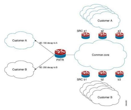
LISP encapsulated data packets that do not carry a valid source RLOC are dropped. The combination of RLOC space URPF enforcement and source RLOC-based decapsulation filtering ensures that it not possible for a source that is not member of a tenant VPN to inject traffic into the VPN.
