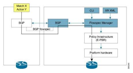
Here, the Controller on the left-hand side injects the flowspec NRLI, and the client on the right-hand side receives the information, sends it to the flowspec manager, configures the ePBR (Enhance Policy-based Routing) infrastructure, which in turn programs the hardware from the underlaying platform in use.
