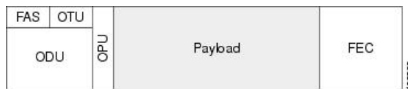
Figure 1: OTN Optical Channel Structure
