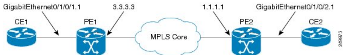
Figure 10: VPLS with BGP autodiscovery and BGP signaling
