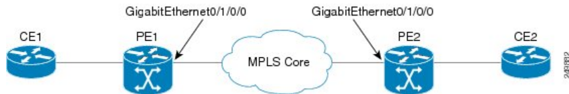
Figure 11: VPLS with BGP autodiscovery and LDP signaling
