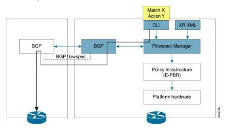
The Controller is configured using CLI to provide that entry for NRLI injection.
