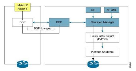
Here, the Controller on the left-hand side injects the flowspec NRLI, and the client on the right-hand side receives the information, sends it to the flowspec manager, configures the ePBR (Enhanced Policy-based Routing) infrastructure, which in turn programs the hardware from the underlaying platform in use.
