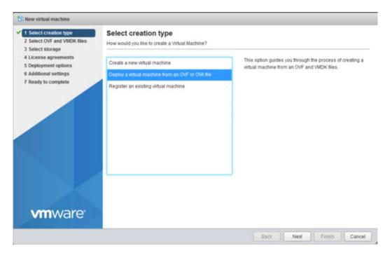
In the Select OVF and VMDK files tab, provide a name for the virtual machine and browse to an OVF package from the internet or a file accessible from your computer (for example, iot-fnd-4.10.0-40.ova). Click **Next**.
