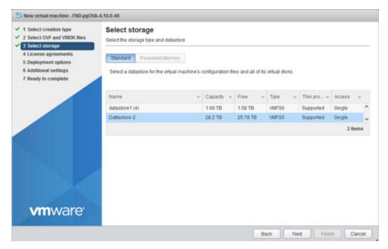
After selecting the data store, select the provisioning type and enable the **Power on automatically** option. This ensures to power on the virtual machine once the deployment process is complete. Click **Next**.
