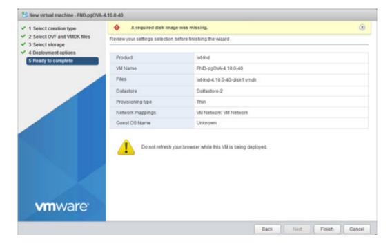
The virtual machine deployment is initiated. After completion of the install, the "Completed successfully" message appears in the Recent tasks pane at the bottom of the install window.
