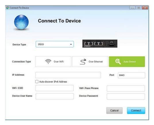
**Step 2** In the Connect to Device dialog box, select the Device Type: **IR809** or **IR829**.
