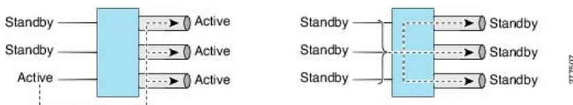
VPLS decoupled mode is when all pseudowires in the VFI are always active and the attachment circuit state is independent of the pseudowire state. This mode provides faster switchover time when a platform does not support pseudowire status functionality, but extra flooding and multicast traffic will be dropped on the PE with standby attachment circuits. However, if the attachment circuit is down, all pseudowires also go down. See the figure below.
