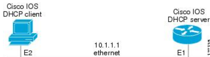
Figure 2: Topology Showing DHCP Client with GigabitEthernet Interface
