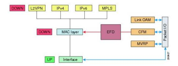
The figure shows CFM detection of an error on one of its sessions EFD signaling an error to the corresponding MAC layer for the interface. This triggers the MAC to go to a down state, which further triggers all higher level protocols (Layer 2 pseudowires, IP protocols, and so on) to go down and also trigger a reconvergence where possible. As soon as CFM detects there is no longer any error, it can signal to EFD and all protocols will once again go active.
