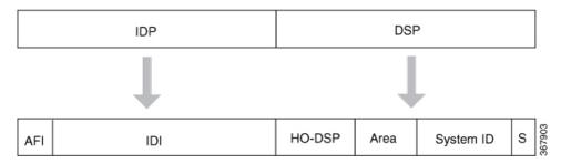
Assign addresses or NETs for your domains and areas. The domain address uniquely identifies the routing domain. All routers within a given domain are given the same domain address. Within each routing domain, you can set up one or more areas, as shown in Figure 2. Determine which routers are to be assigned to which areas. The area address uniquely identifies the routing area and the system ID identifies each node.
