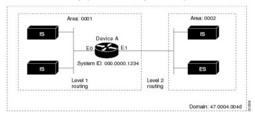
The key difference between the ISO IGRP and IS-IS NSAP addressing schemes is in the definition of area addresses. Both use the system ID for Level 1 routing (routing within an area). However, they differ in the way addresses are specified for area routing. An ISO IGRP NSAP address includes three separate fields for routing: the domain, area, and system ID. An IS-IS address includes two fields: a single continuous area field (comprising the domain and area fields) and the system *ID*.
