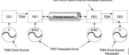
Differential timing messages are used to tune the TDM clock frequency from the sending end to the receiving end.
