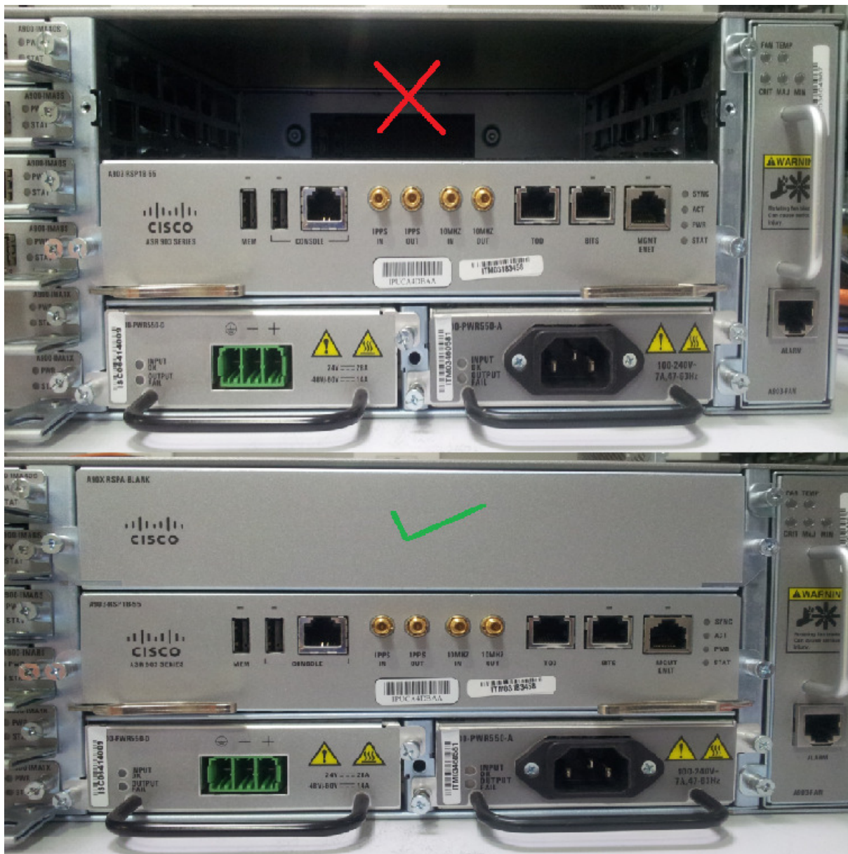
Figure 7: Empty Slots Must be Filled with Blank Fillers
