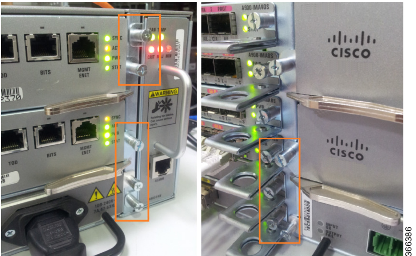
Figure 5: Tighten All Captive Screws
