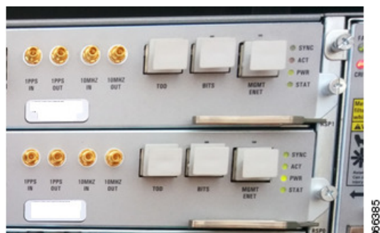
Figure 4: Closing Unused Ports with Protective Dust Caps
