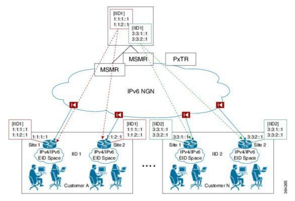
In the example, the Map-Servers build a separate VPN (EID instance) membership list for each customer and then push the contents of the list out. The two xTRs for customer A each register their site RLOCs. They each receive back from the Map-Server the complete list of RLOCs of all the xTRs for customer A. The received list is used to filter decapsulated traffic and enforce the data plane security.
