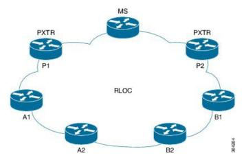
As an example consider the network in the above figure with two VPNs. VPNs A and B each have two xTRs A1/A2 and B1/B2 respectively. The membership of VPN A is extended on the MS through the "map-server rloc members add …" configuration to include PxTR RLOC address P1. The membership of VPN B is extended to include PxTR RLOC address P2. The resulting lists maintained by the MS are:
