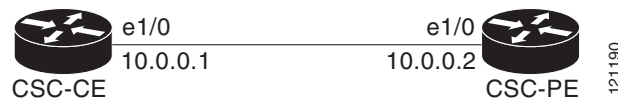
Figure 6 Configuration for Peering with Directly Connected Interfaces Between CSC-PE and CSC-CE Routers
