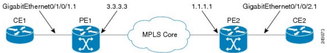
Figure 20: VPLS with BGP autodiscovery and BGP signaling
