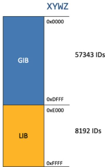
With this allocation scheme, the uSID Block **FCBB:BB00::/32** supports up to 57343 global uSIDs (routers) with each router supporting up to 8192 local uSIDs.
