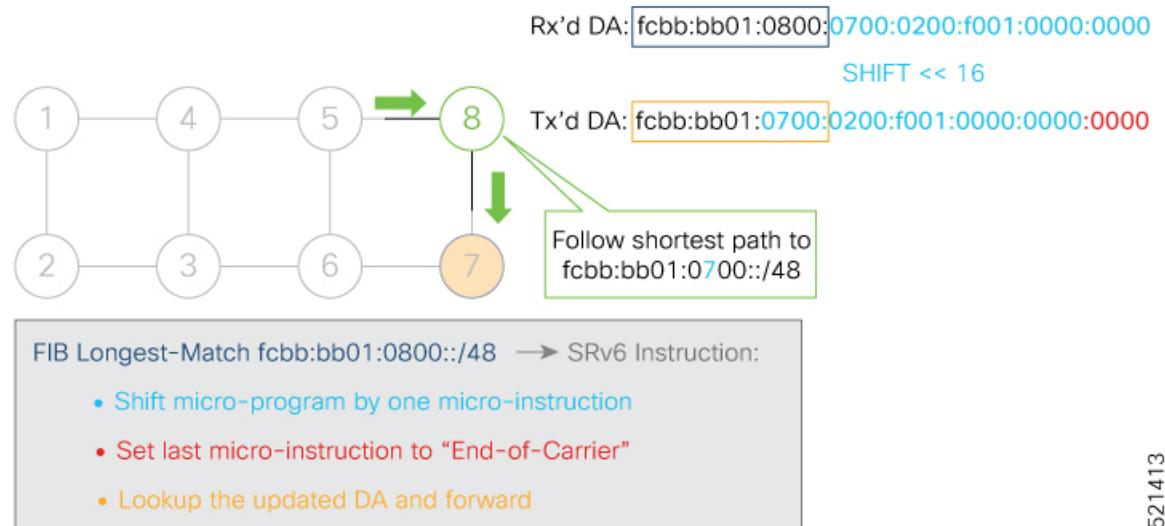
When Node 7 receives the packet, it performs the same SRv6 uN behavior (shift-and-lookup with PSP/USD), forwarding it using the new DA fcbb:bb01:**0200**:f001:0000:0000:0000:0000
