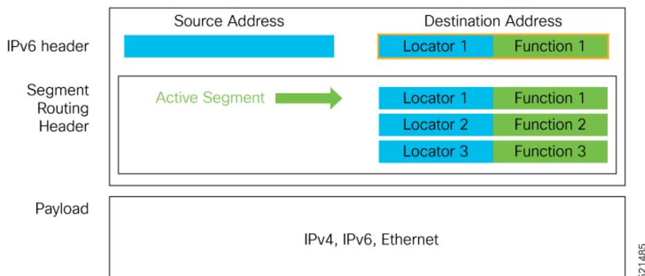
The SRv6 SRH is documented in IETF RFC [IPv6 Segment Routing Header \(SRH\)](#).
