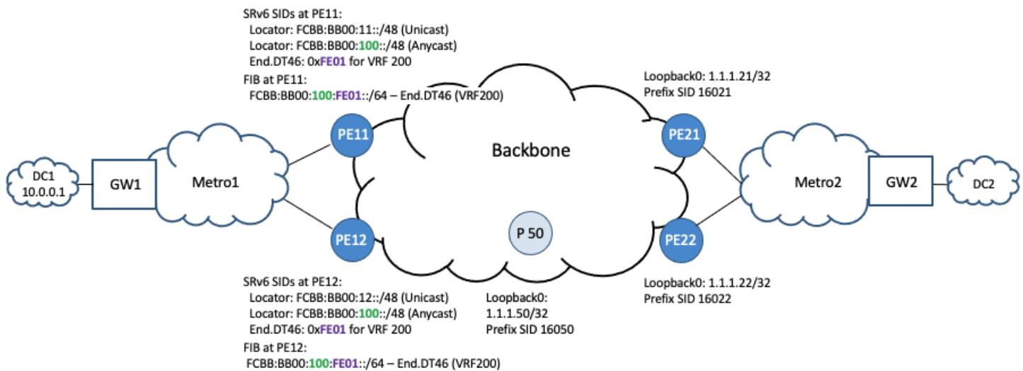
The SRv6 PE lite nodes are configured with SRv6 locators and explicit (manually assigned) service de-multiplexing end-point behaviors to perform decapsulation and VPN table lookup.
