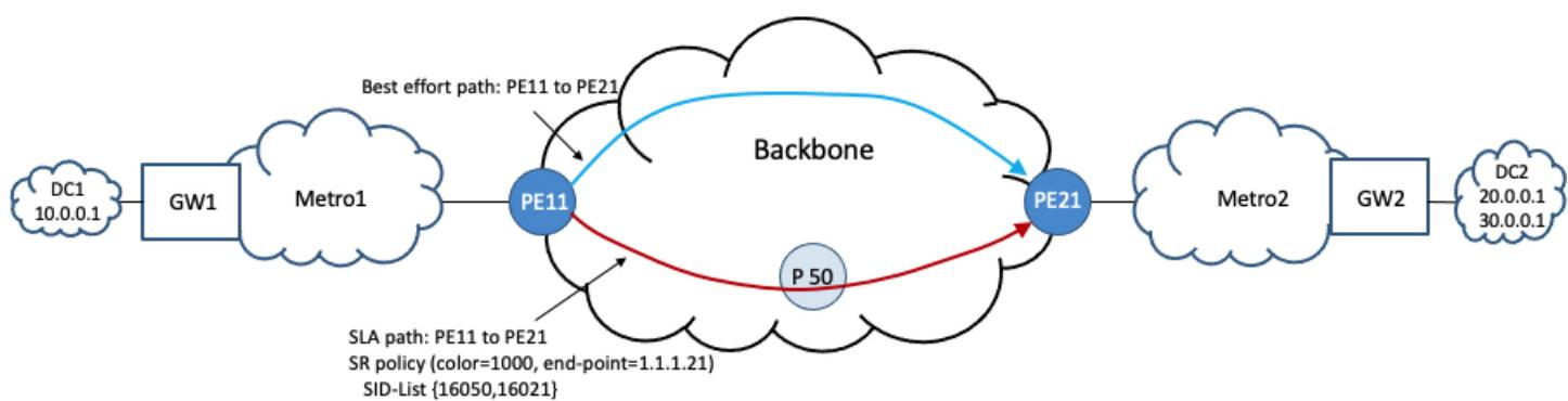
For traffic in the direction DC1 to DC2, the SRv6 PE lite node PE11 is an SR-TE headend of an SR policy associated with color 1000 and end-point of PE21. This SR policy will be used to steer traffic toward BGP service routes with color 1000 advertised by PE21. As an example, this SR policy is associated with a segment list that includes the prefix SID of a transit router in the backbone (PE50) and the prefix SID of the intended egress PE (PE21).
