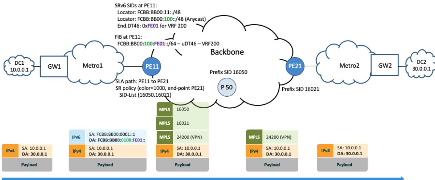
Traffic arriving at GW1 destined for 30.0.0.1 in DC2 is encapsulated into an outer IPv6 header with a destination address of FCBB:BB00:100:FE01::. As in the previous case, this address is composed of the Anycast locator at PE11 and the explicit End.DT46 function value of VRF 200. Any transit nodes in the Metro1 domain simply perform a longest-prefix-match lookup for prefix FCBB:BB00:100::/48 and forward the packet along the shortest path to PE11.
