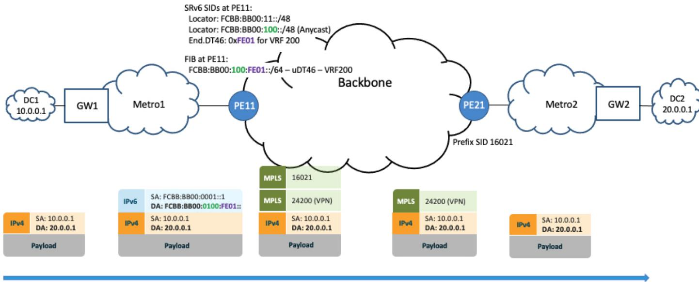
Traffic arriving at GW1 destined for 20.0.0.1 in DC2 is encapsulated into an outer IPv6 header with a destination address of FCBB:BB00:100:FE01::. This address is composed of the Anycast locator at PE11 and the explicit End.DT46 function value of VRF 200. Any transit nodes in the Metro1 domain simply perform a longest-prefix-match lookup for prefix FCBB:BB00:100::/48 and forward the packet along the shortest path to PE11.
