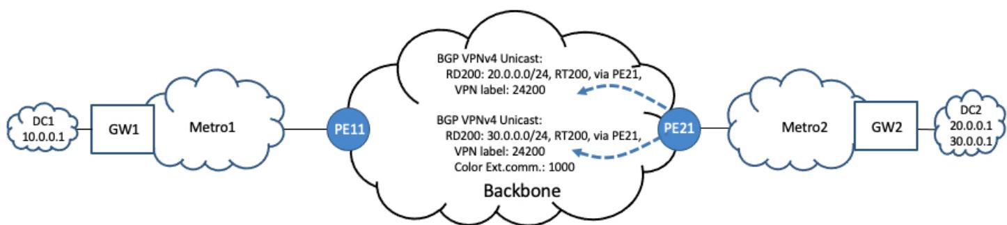
Prefixes from the data center are advertised in the backbone via multiprotocol BGP as part of a VPN. These prefixes can include a color extended community in order to indicate the desired transport SLA. For example, PE21 advertises BGP VPN overlay routes for DC2, 20.0.0.0/24 and 30.0.0.0/24. Prefix 20.0.0.0/24 requires best-effort treatment. Prefix 30.0.0.0/24 requires a transport SLA indicated by the presence of color extended community of value 1000.
