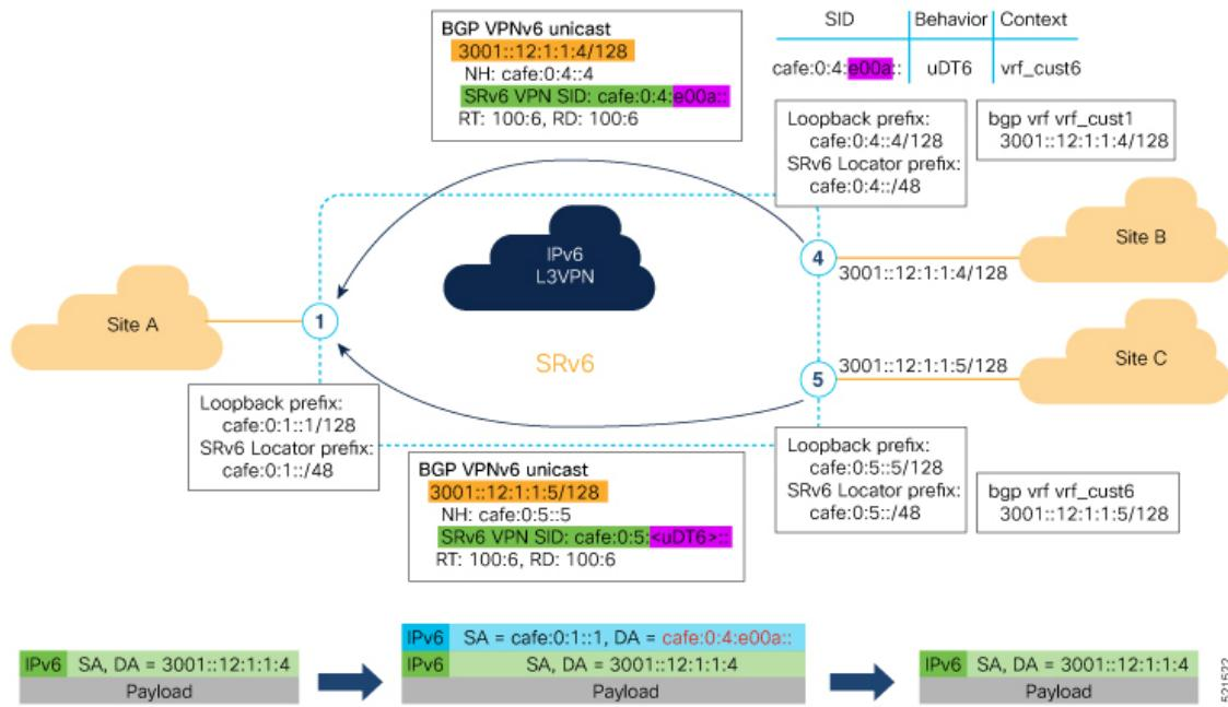
The following examples shows how to verify the SRv6 based L3VPN configurations for an Individual VRF with per VRF label allocation mode.
