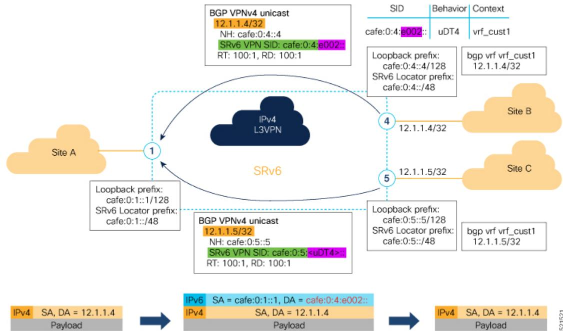
The following example shows how to verify the SRv6 based L3VPN configuration using the **show segment-routing srv6 sid** command.
