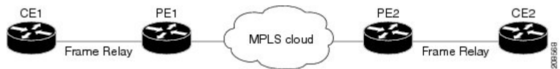
Figure 8: Frame Relay Over MPLS
