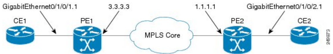
Figure 20: VPLS with BGP autodiscovery and BGP signaling
