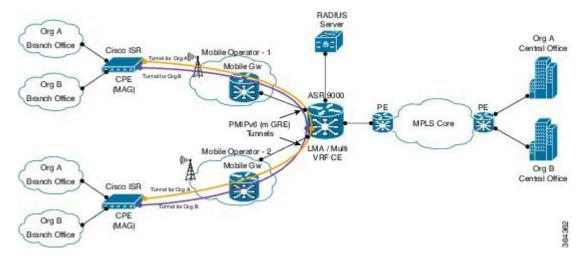
The following figure is a sample topology of Mobile Local Loop service hosted on MPLS Provider Edge (PE) routers:
