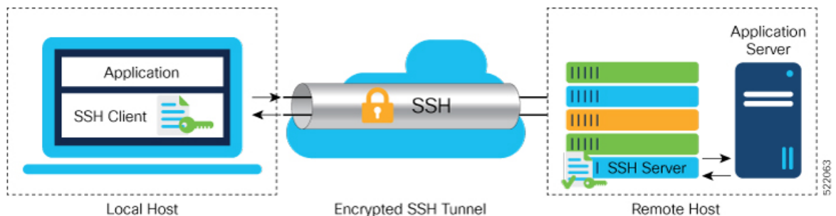
Figure 1: SSH Port Forwarding
