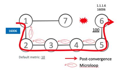
With microloop avoidance configured on Node1, a post-convergence path is computed and possible microloops on the post-convergence path for any destination are detected.
