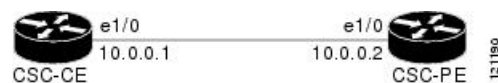
Figure 7: Configuration for Peering with Directly Connected Interfaces Between CSC-PE and CSC-CE Routers
