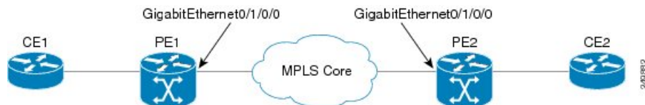
Figure 39: VPLS with BGP autodiscovery and LDP signaling
