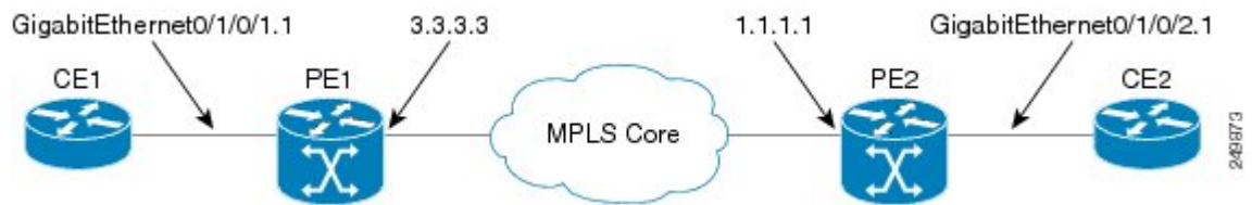
Figure 38: VPLS with BGP autodiscovery and BGP signaling
