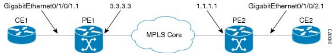
Figure 38: VPLS with BGP autodiscovery and BGP signaling
