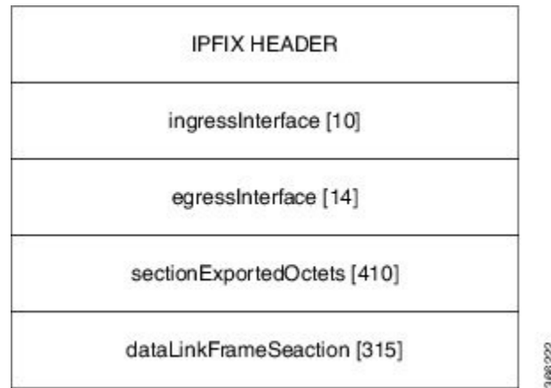
Figure 4: IPFIX 315 Export Packet Format
