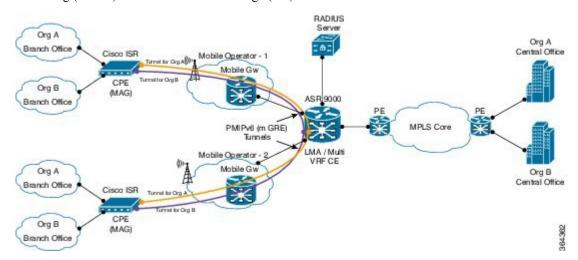
The following figure is a sample topology of Mobile Local Loop service hosted on MPLS Provider Edge (PE) routers:
