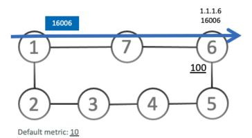
TI-LFA on Node7 pre-computes a backup path for traffic to Node6 (prefix SID 16006) that will be activated if the link between Node7 and Node6 goes down. In this network, the backup path would steer traffic toward Node5 (prefix SID 16005) and then via link between Node5 and Node6 (adj-SID 24056). All nodes are notified of the topology change due to the link failure.
