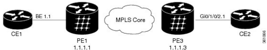
Figure 11: PBB-EVPN on Single Homed Device/Single Homed Network
