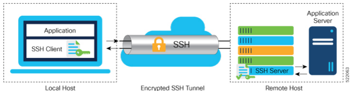
Figure 15: SSH Port Forwarding
