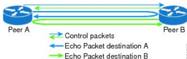
Figure 2: BFD Asynchronous Mode With Echo Packets
